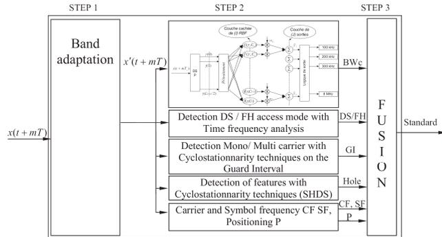
Figure 3. The new standard recognition sensor.
