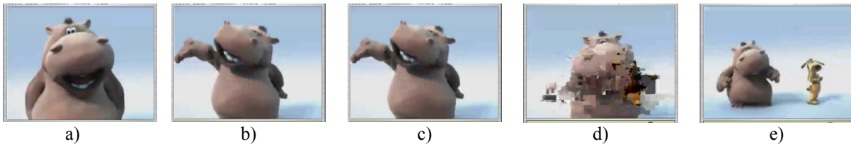
Figure 6. Video snapshots at: a) 450s (before congestion), b) 470s (congestion beginning), c) 480s (frozen image), d) 520s (distortion), e) 550s (recuperated image).
