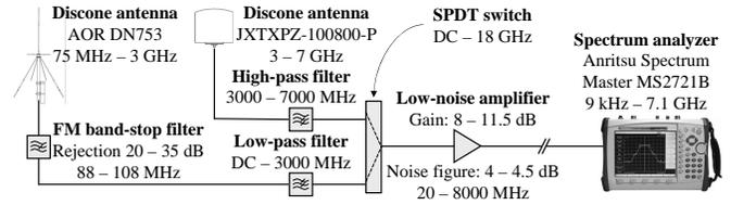
Fig. 1. Measurement setup employed in this study.
