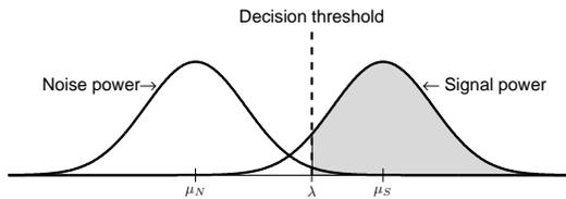
Fig. 7. Model considered for computing the duty cycle (shaded area).
